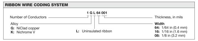
The Wire and Cable Coding System shown above gives the unique designation of each wire type for ordering purposes. The leadwire and cabling selection charts presented on the next three pages are organized according to the number of conductors. All wires and cables are supplied on spools for user convenience. Some styles may not be continuous length.
